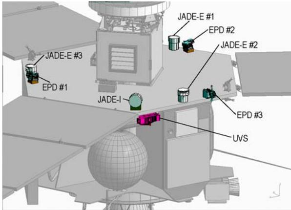
Fig. 12: Deck-mounted instruments simplify integration and test.
