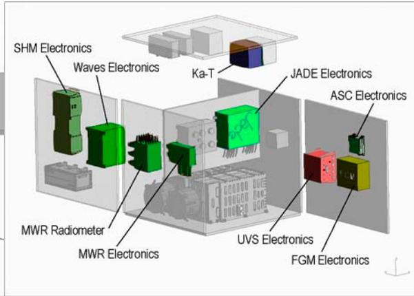
Fig. 13: Vault protects instruments from radiation.
