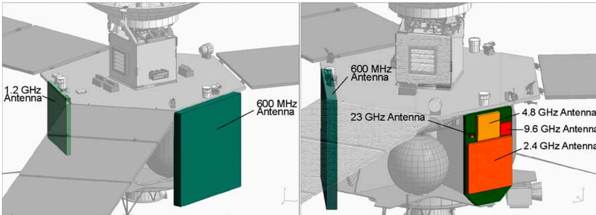
Fig. 14: MWR antennas are mounted to maximize FOV.
