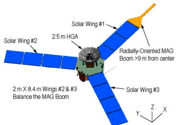
Fig. 17: Spinning S/C provides stability, accurate pointing, and simple operations.
