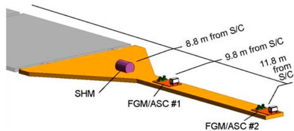
Fig. 15: Radial separation of FGM sensors on MAG Boom improves measurement of S/C magnetic fields. S/C fields are greatly reduced by >8.8m distance.
