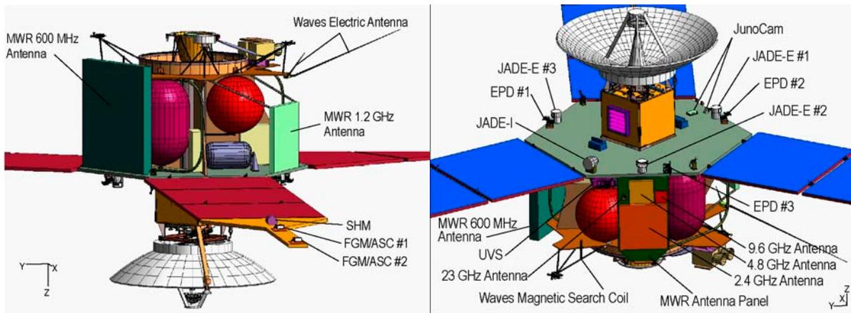
Fig. 11: Spacecraft design fully accommodates all science instrument requirements.
